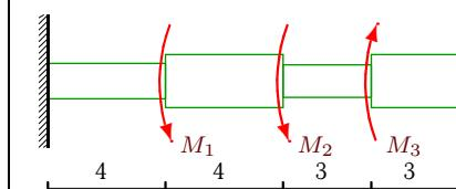
$$M_1 = 56\text{kNm}, M_2 = 32\text{kNm}, M_3 = 16\text{kNm}, d_1 = 0.12\text{м}, d_2 = 0.18\text{м}, d_3 = 0.11\text{м}, d_4 = 0.18\text{м}.$$
