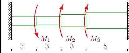
$$M_1 = 7\text{kNm}, M_2 = 18\text{kNm}, M_3 = 44\text{kNm}, d_1 = 0.11\text{м}, d_2 = 0.1\text{м}, d_3 = 0.15\text{м}, d_4 = 0.19\text{м}.$$
