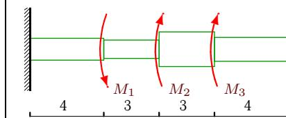
$$M_1 = 9\text{kNm}, M_2 = 6\text{kNm}, M_3 = 52\text{kNm}, d_1 = 0.12\text{м}, d_2 = 0.1\text{м}, d_3 = 0.19\text{м}, d_4 = 0.13\text{м}.$$
