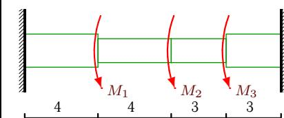
$$M_1 = 24\text{kNm}, M_2 = 20\text{kNm}, M_3 = 7\text{kNm}, d_1 = 0.18\text{м}, d_2 = 0.13\text{м}, d_3 = 0.13\text{м}, d_4 = 0.18\text{м}.$$
