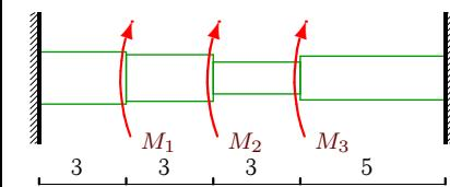
$$M_1 = 24\text{kNm}, M_2 = 36\text{kNm}, M_3 = 6\text{kNm}, d_1 = 0.18\text{м}, d_2 = 0.16\text{м}, d_3 = 0.11\text{м}, d_4 = 0.15\text{м}.$$
