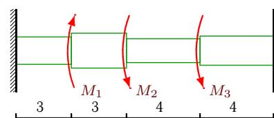
$$M_1 = 10\text{kNm}, M_2 = 7\text{kNm}, M_3 = 24\text{kNm}, d_1 = 0.15\text{м}, d_2 = 0.19\text{м}, d_3 = 0.13\text{м}, d_4 = 0.16\text{м}.$$
