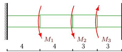
$$M_1 = 48\text{kNm}, M_2 = 18\text{kNm}, M_3 = 6\text{kNm}, d_1 = 0.14\text{м}, d_2 = 0.16\text{м}, d_3 = 0.16\text{м}, d_4 = 0.14\text{м}.$$
