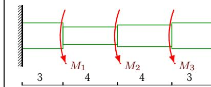
$$M_1 = 7\text{kNm}, M_2 = 55\text{kNm}, M_3 = 9\text{kNm}, d_1 = 0.19\text{м}, d_2 = 0.13\text{м}, d_3 = 0.16\text{м}, d_4 = 0.19\text{м}.$$
