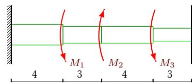
$$M_1 = 12\text{kNm}, M_2 = 44\text{kNm}, M_3 = 10\text{kNm}, d_1 = 0.16\text{м}, d_2 = 0.13\text{м}, d_3 = 0.13\text{м}, d_4 = 0.1\text{м}.$$
