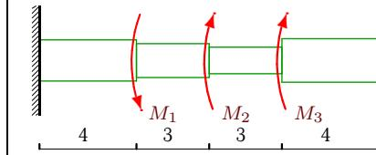
$$M_1 = 35\text{kNm}, M_2 = 18\text{kNm}, M_3 = 52\text{kNm}, d_1 = 0.17\text{м}, d_2 = 0.14\text{м}, d_3 = 0.11\text{м}, d_4 = 0.18\text{м}.$$
