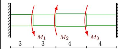
$$M_1 = 7\text{kNm}, M_2 = 36\text{kNm}, M_3 = 12\text{kNm}, d_1 = 0.15\text{м}, d_2 = 0.14\text{м}, d_3 = 0.17\text{м}, d_4 = 0.14\text{м}.$$
