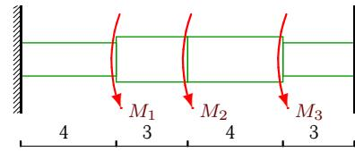
$$M_1 = 50\text{kNm}, M_2 = 7\text{kNm}, M_3 = 24\text{kNm}, d_1 = 0.14\text{м}, d_2 = 0.19\text{м}, d_3 = 0.19\text{м}, d_4 = 0.14\text{м}.$$
