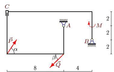
$$P = 40 \text{ кН}, Q = 50 \text{ кН}, \alpha = 60^\circ, \beta = 45^\circ, \rho = 2 \text{ кН/м}, M = 10 \text{ кНм}.$$
