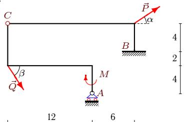
$$P = 10 \text{ kH}, Q = 20 \text{ kH}, \alpha = 30^\circ, \beta = 60^\circ, \rho = 5 \text{ kH/m}, M = 30 \text{ kNm}.$$
