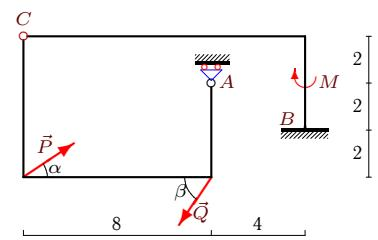
$$P = 10 \text{ кН}, Q = 20 \text{ кН}, \alpha = 30^\circ, \beta = 60^\circ, \rho = 5 \text{ кН/м}, M = 10 \text{ кНм}.$$
