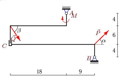
$$P = 60 \text{ kH}, Q = 70 \text{ kH}, \alpha = 45^\circ, \beta = 60^\circ, \rho = 2 \text{ kH/m}, M = 100 \text{ kNm}.$$
