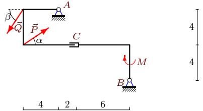
$$P = 10 \text{ kH}, Q = 20 \text{ kH}, \alpha = 30^\circ, \beta = 60^\circ, \rho = 2 \text{ kH/m}, M = 80 \text{ kNm}.$$
