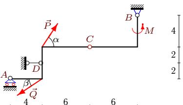
$P = 20 \text{ kH}$ ,  $Q = 30 \text{ kH}$ ,  $\alpha = 60^\circ$ ,
