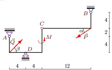
$$P = 30 \text{ kH}, Q = 40 \text{ kH}, \alpha = 30^\circ, \beta = 45^\circ, \rho = 3 \text{ kH/m}, M = 50 \text{ kNm}.$$
