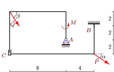
$$P = 10 \text{ кН}, Q = 20 \text{ кН}, \alpha = 30^\circ, \beta = 60^\circ, \rho = 6 \text{ кН/м}, M = 110 \text{ кНм}.$$
