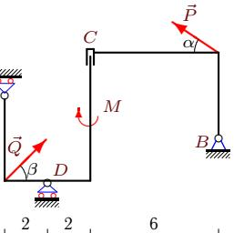
$$P = 30 \text{ кН}, Q = 40 \text{ кН}, \alpha = 30^\circ, \beta = 45^\circ, \rho = 4 \text{ кН/м}, M = 50 \text{ кНм}.$$
