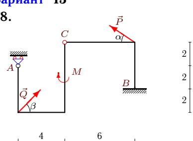
$P = 30 \text{ kH}$ ,  $Q = 40 \text{ kH}$ ,  $\alpha = 30^\circ$ ,
