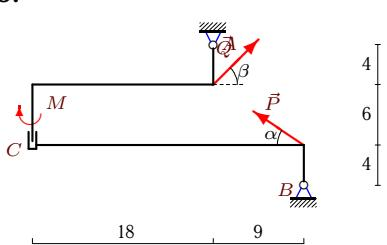
$$P = 30 \text{ kH}, Q = 40 \text{ kH}, \alpha = 30^\circ, \beta = 45^\circ, \rho = 2 \text{ kH/m}, M = 110 \text{ kNm}.$$
