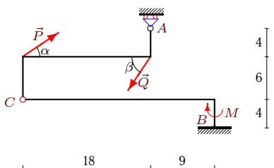
$P = 10 \text{ kH}$ ,  $Q = 20 \text{ kH}$ ,  $\alpha = 30^\circ$ ,
