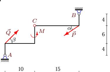
$$P = 30 \text{ kH}, Q = 40 \text{ kH}, \alpha = 30^\circ, \beta = 45^\circ, \rho = 1 \text{ kH/m}, M = 60 \text{ kNm}.$$
