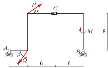
$$P = 10 \text{ кН}, Q = 20 \text{ кН}, \alpha = 30^\circ, \beta = 60^\circ, \rho = 2 \text{ кН/м}, M = 50 \text{ кНм}.$$
