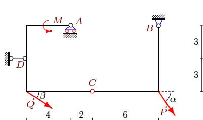
$P = 20 \text{ kH}$ ,  $Q = 30 \text{ kH}$ ,  $\alpha = 60^\circ$ ,
