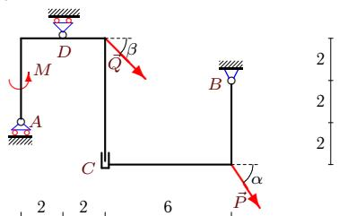
$$P = 40 \text{ кН}, Q = 50 \text{ кН}, \alpha = 60^\circ, \beta = 45^\circ, \rho = 4 \text{ кН/м}, M = 130 \text{ кНм}.$$
