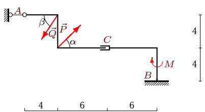
$$P = 60 \text{ kH}, Q = 70 \text{ kH}, \alpha = 45^\circ, \beta = 60^\circ, \rho = 6 \text{ kH/m}, M = 70 \text{ kNm}.$$
