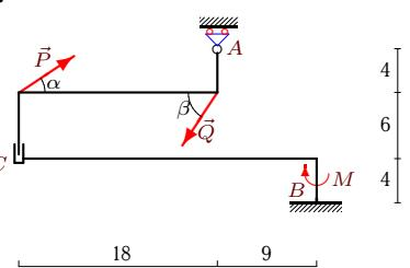
$$P = 10 \text{ kH}, Q = 20 \text{ kH}, \alpha = 30^\circ, \beta = 60^\circ, \rho = 6 \text{ kH/m}, M = 90 \text{ kNm}.$$
