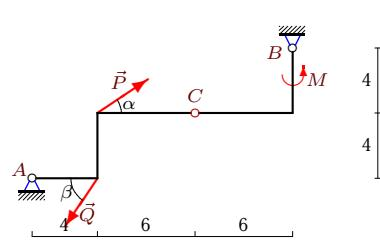
$$P = 10 \text{ кН}, Q = 20 \text{ кН}, \alpha = 30^\circ, \beta = 60^\circ, \rho = 1 \text{ кН/м}, M = 50 \text{ кНм}.$$
