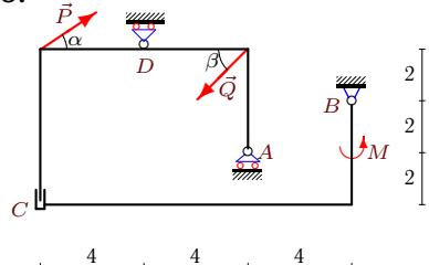
$P = 30 \text{ kH}$ ,  $Q = 40 \text{ kH}$ ,  $\alpha = 30^\circ$ ,
