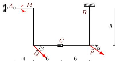
$P = 30 \text{ kH}$ ,  $Q = 40 \text{ kH}$ ,  $\alpha = 30^\circ$ ,
