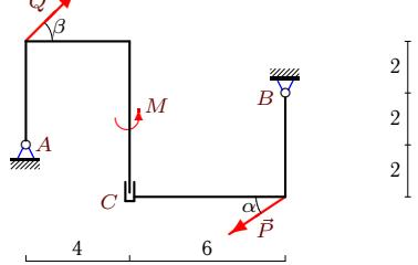
$$P = 30 \text{ кН}, Q = 40 \text{ кН}, \alpha = 30^\circ, \beta = 45^\circ, \rho = 2 \text{ кН/м}, M = 140 \text{ кНм}.$$
