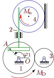
$$\begin{aligned}M_{Dz} &= M_0 - k\omega_{1z}, \quad M_{n_z} = -\mu\omega_{4z}, \\&\varphi_{1,0} = 1.2, \quad \omega_{1z,0} = 0.3\frac{1}{c}, \\M_0 &= 11 \text{ Нм}, \quad k = 13 \text{ Нмс}, \\&\mu = 13 \text{ Нмс}, \\I_1 &= 11 \text{ кгм}^2, \quad m_2 = 15 \text{ кг}, \quad m_3 = 33 \text{ кг}, \\m_4 &= 25 \text{ кг}, \quad R_1 = 36 \text{ см}, \quad r_1 = 25 \text{ см}, \\R_3 &= 26 \text{ см}, \quad R_4 = 20 \text{ см}, \quad r_4 = 12 \text{ см}, \quad i_4 = 14 \text{ см.}\end{aligned}$$
