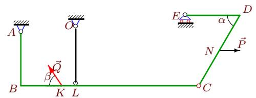
$P = 8 \text{ кН}$ ,  $Q = 8 \text{ кН}$ ,  $\alpha = 60^\circ$ ,  $\beta = 75^\circ$ ,
